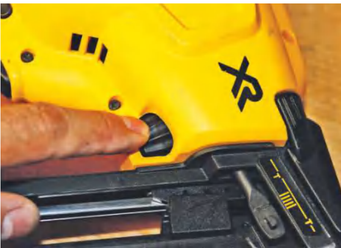
▲ Depth of drive is set with this dial, reading the position on the nose indicator
